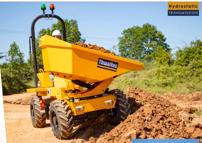
The Thwaites 2.3 Tonne Power Swivel, Stage V dumper is manufactured with contractors and hirers in mind – ensuring operator safety, reducing risk on site and improving performance. Powered by an 18.4 kW 3-cylinder Yanmar engine, delivering 107 Nm max torque for optimum traction and control, this machine is driven by a Hydrostatic transmission, making it simple and straightforward to operate.
